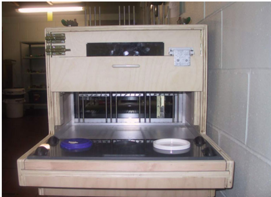
Fig. 1. (colour online) Test apparatus for cognitive assessment of felines. The apparatus consists of an enclosure where the cat was placed for 5–15 min during the cognitive test and a sliding tray with three food wells.
